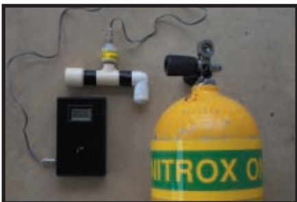
Photo 1 —I built the Nitrox analyzer because of my interest in both embedded systems and scuba diving. Here you see the analyzer along with the oxygen sensor in the PVC sensor mount and a tank of Nitrox.
