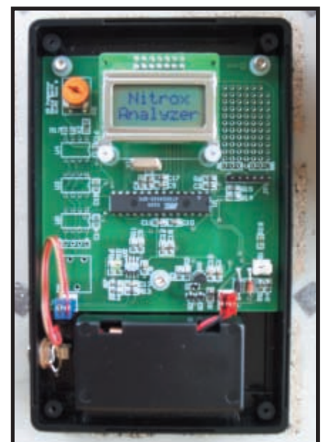
Photo 2 —Take a look at the Nitrox Analyzer's main electronic components, subsystems, and PCB. Note the homemade protoboard section in the upper right corner.
